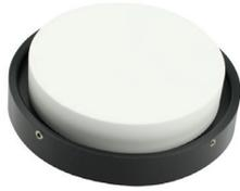
Integrating sphere port plugs are used to block an unused port on the sphere. They are offered in PTFE, barium sulfate (Spectrafect), diffuse gold, or flat black for various port sizes. In case the right size port plug is not available, consider first mounting a port reducer and then a right size port plug.
